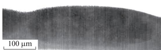
**Fig. 3.** HAADF STEM image of the elliptical domain in the PTB7:PC<sub>71</sub>BM photoactive layer cross section.
